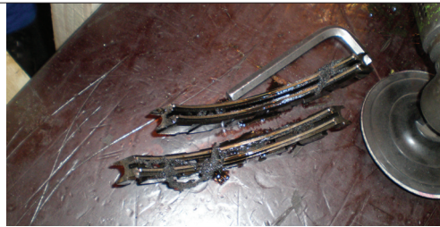
A stuffing box with damage caused by cat fines
